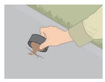
4. Fill the crack with a concrete crack sealer available at any home care center, following the manufacturer's instructions. Overfill the crack slightly to allow for shrinkage.
