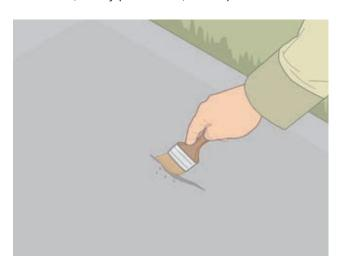
3. Measure the depth of the crack. If it is deeper than ½ inch, fill up the crack with sand or backer rod to within ¼ inch of the surface. If the crack isn't deeper than ½ inch, just move on to the next step.
